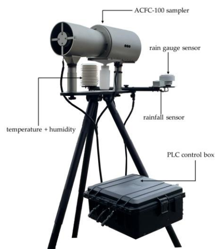
Figure 1. Complete view of the ACFC. Above the PLC control box with a platform anchored by a tripod and the sampler with automatic baffle, plus the sensor module.
